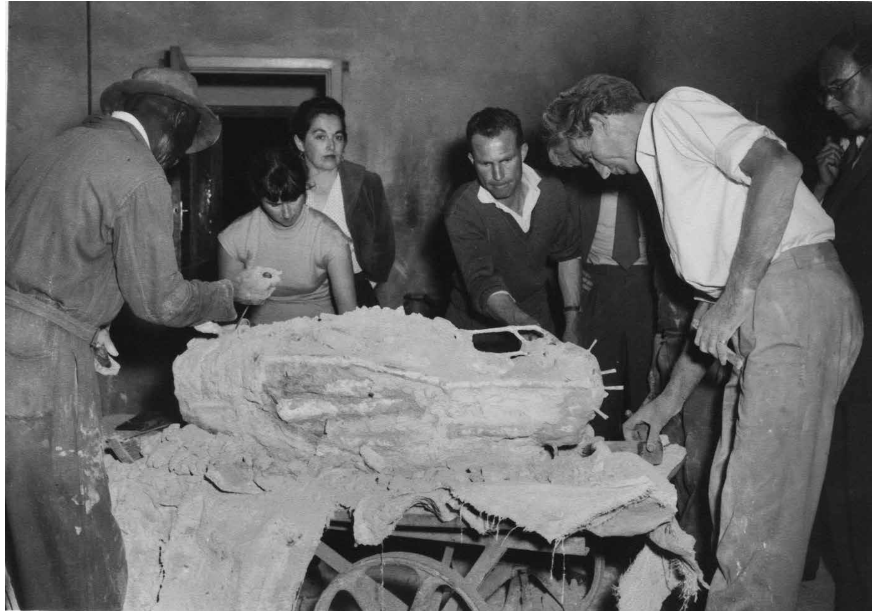
The final plaster mold is now smashed till the bronze core is revealed. It is still extremely hot
