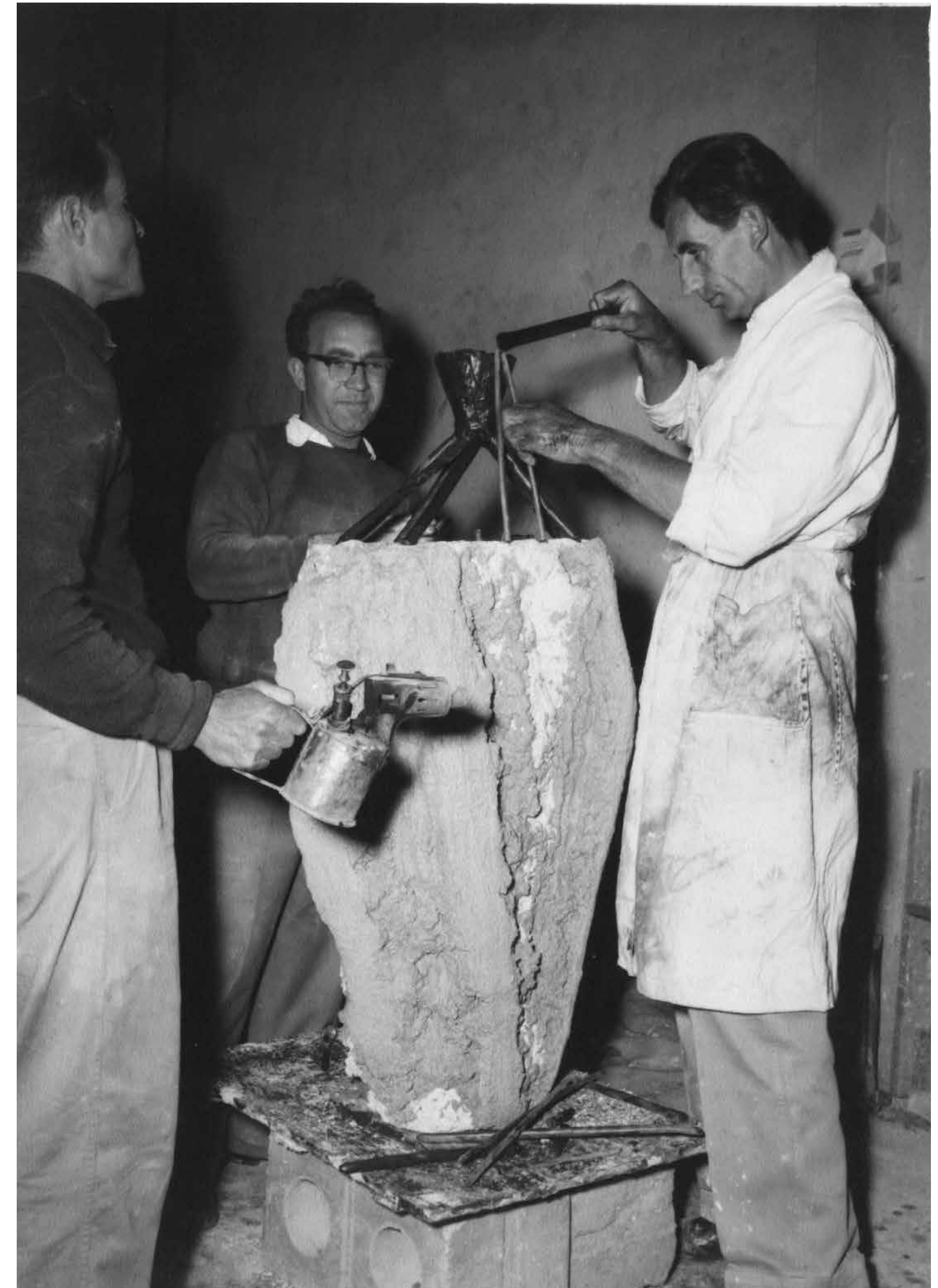
Constructing the funnel form which directs molten bronze into the main mold.
