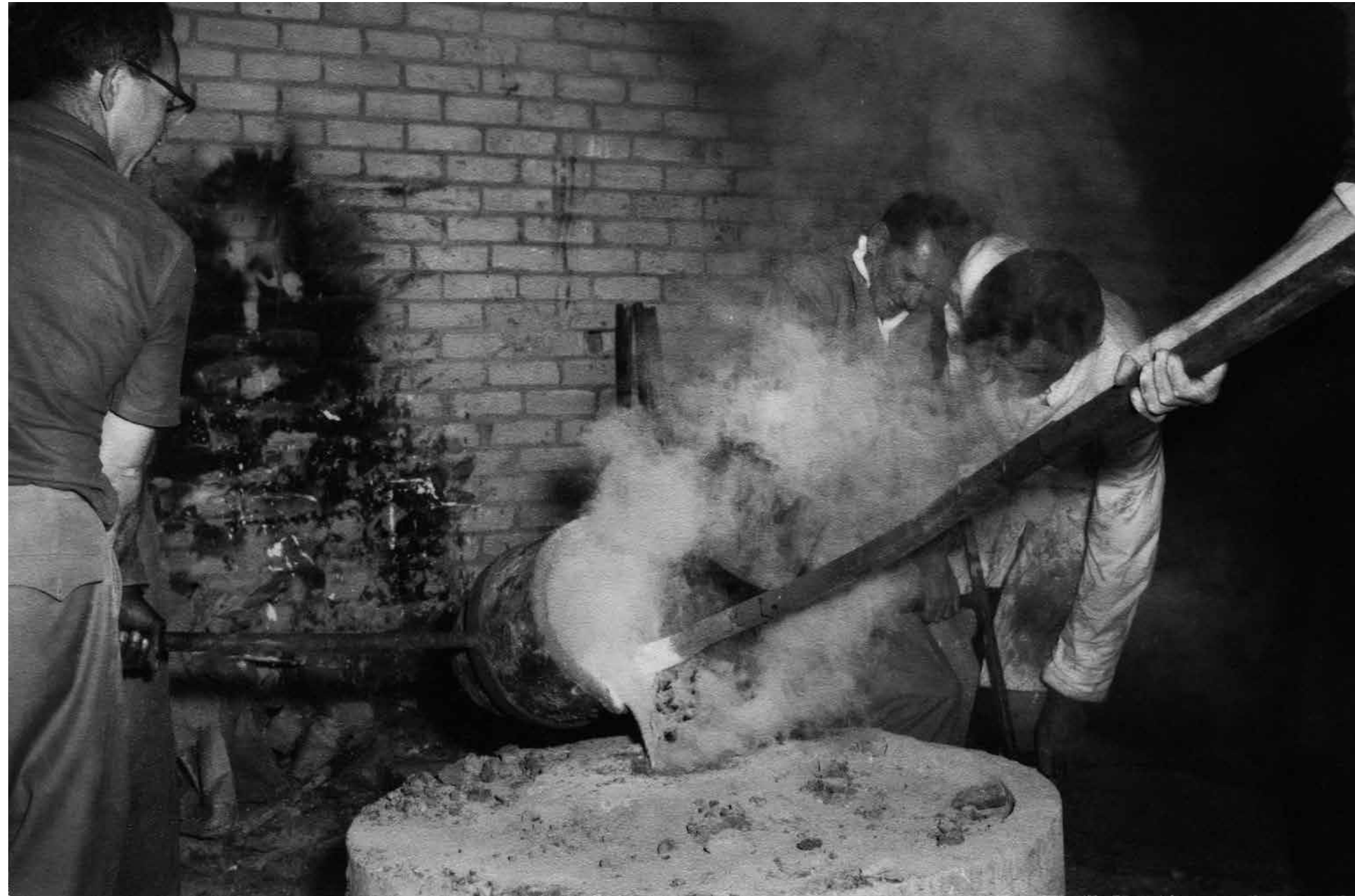
Molten bronze is carefully poured from the crucible into the semi buried final plaster mold. The mold must be totally dry. Any moisture could turn to steam may not vent and this could cause gaps in the cast. In a worst case scenario high pressure steam which could cause molten bronze explode and injure those who are present and pouring.
