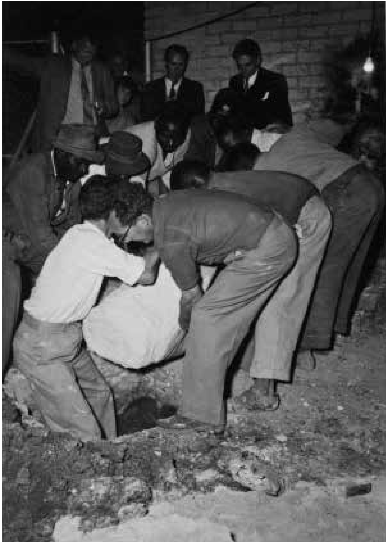
The bronze has cooled and solidified and the entire mold is removed from the ground.
