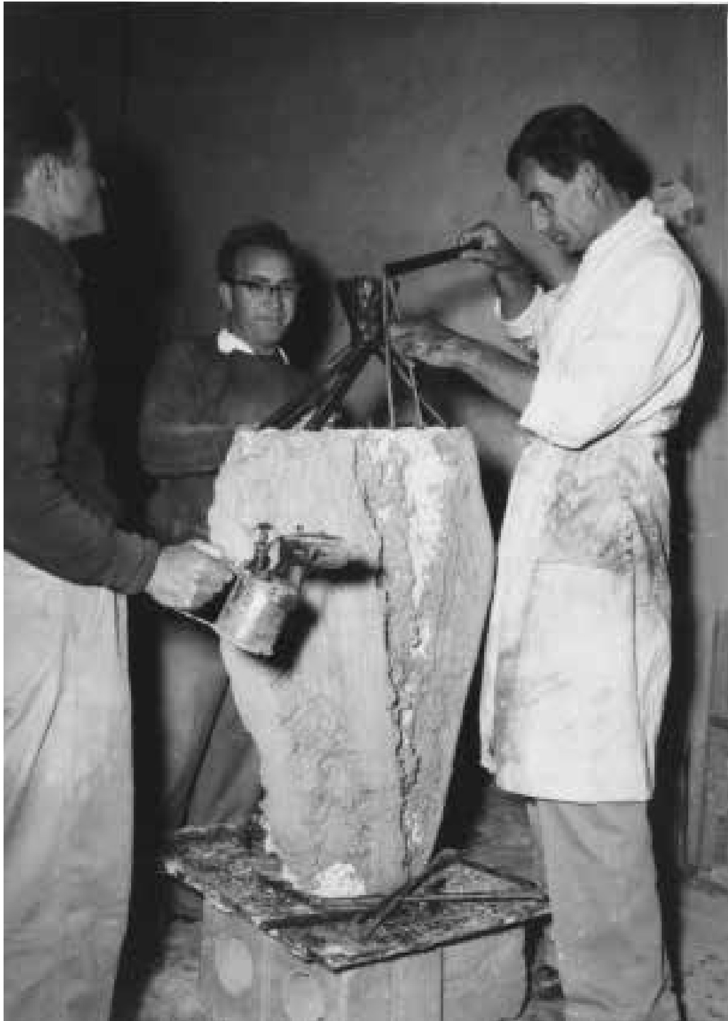
Constructing the funnel form which directs molten bronze into the main mold.
