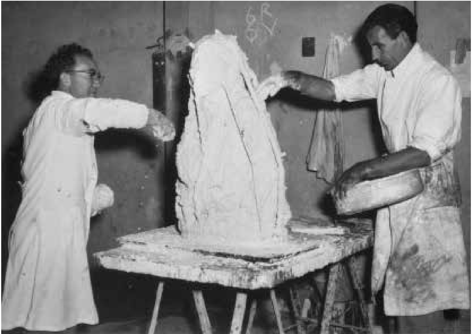
The wax model with a fireproof suspended core, all enclosed by the final outer mold will be baked in the oven till the wax vaporizes, leaving a void which will be filled with molten bronze.
